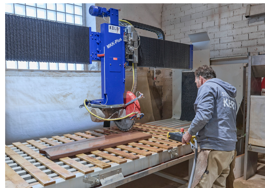
Top: The remote control speeds up the positioning of the saw.
