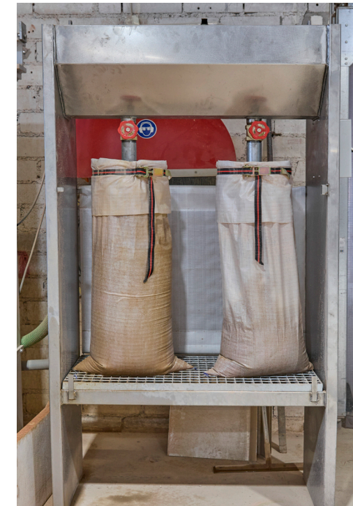
Right: The dried sludge retained in the filter bags can be disposed of in landfill.
