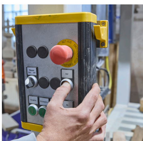
Top: The remote control speeds up the positioning of the saw.
