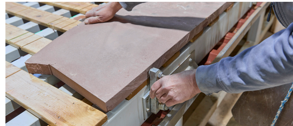
Bottom: The foldable angle stop is a practical detail.
