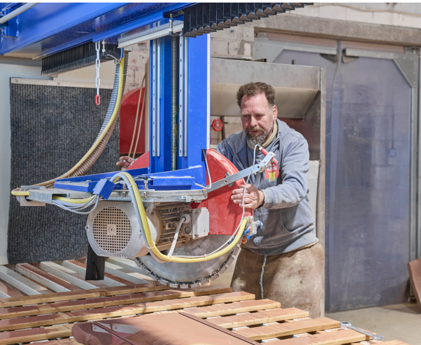
Top: The saw head can be manually swivelled through 90 degrees.
